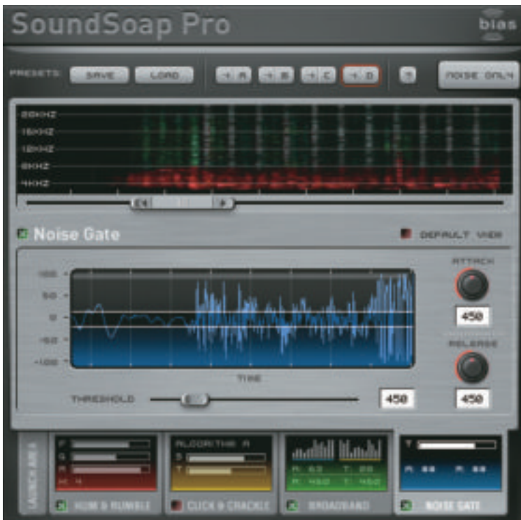
Getting to grips with the noise gate is easy, but it may involve a little experimentation. The two horizontal lines act as gate threshold indicators, controlled via the Threshold slider.
